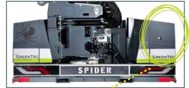
The 220 liter hydraulic tank is located on the right side, and the hydraulic valves and oil cooler are located on the left side.
