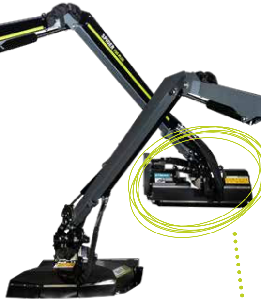
The arm is controlled from the cabin and can be moved from the right to left side and into the driver's field of vision.
